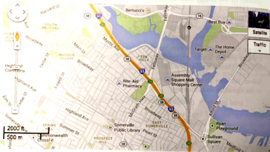
FIGURE 3.1 The miniruler at the lower left acts as the map scale. In this case, the length of the upper segment represents 2000 feet in the city, while the slightly shorter lower segment represents 500 meters.
